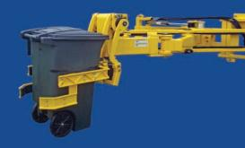
The Perkins Automated Sideloader (PAS) allows the conversion of most drop-frame manual sideloaders into a fully-automated residential collector. This joystick control-based system can retrofit to your existing trucks, automating your fleet within a two-day installation time...at a fraction of the cost that you might expect. Full automation is now within reach.
