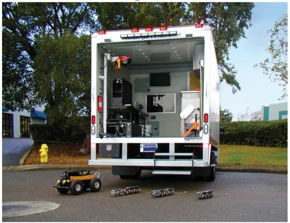
Mounted on the chassis of your choice, the MES **High Cube Truck** is designed for ease and accessibility throughout. The interior is divided into two areas: an operator control room with a passenger door or walk-through into the drivers area, and an equipment room outfitted with a tool cabinet, work bench and efficient storage compartments for system accessories.
