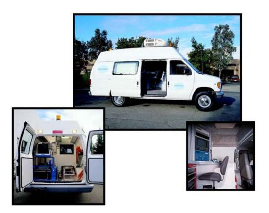
The streamlined design of the **Standard Van** from MES allows ease and accessibility throughout. The interior is divided into three areas: a driver area, operator control room with a tool cabinet and outside door, and an equipment room outfitted with space saving storage compartments for system accessories.
