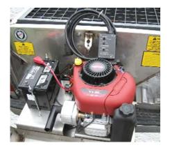
Gas Engine and Cab Controls Equipped with a standard 11.5 HP Briggs & Stratton engine that is fully enclosed to provide protection during loading and operation. In cab controls provide operational controls for ignition, choke, electric throttle and electric clutch.
