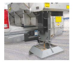
Spinner Assembly Spinner assembly is easily removed between storms or for flat storage in summer. No tools required.
